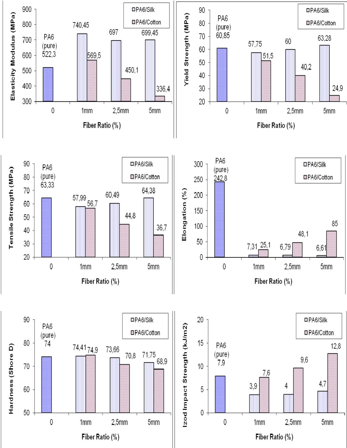
Figure 1 Mechanical properties of the PA<sub>6</sub>/waste silk and PA<sub>6</sub>/waste cotton polymer composites
