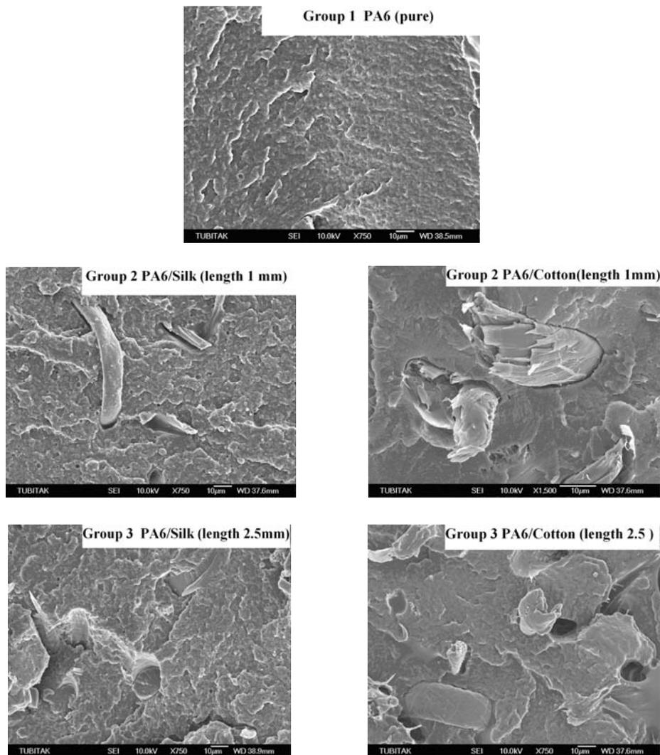
Figure 4 SEM photographs of recycled PA<sub>6</sub>/waste silk & cotton polymer composites
