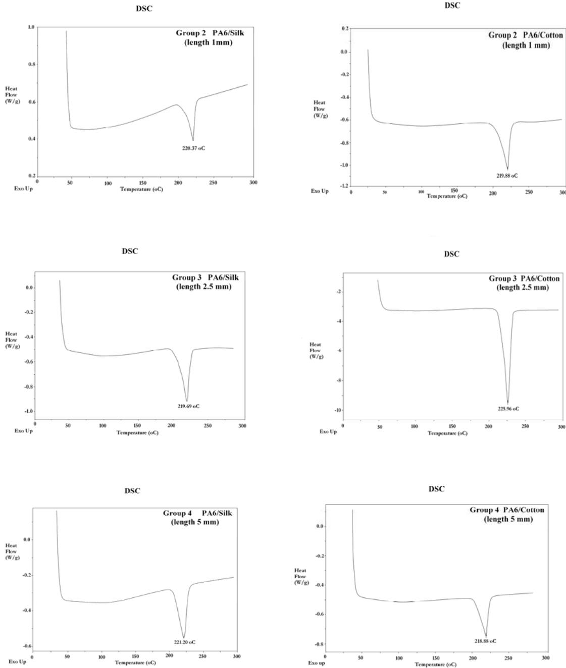
Figure 3 DSC curves of the recycled PA<sub>6</sub>/waste silk and PA<sub>6</sub>/waste cotton polymer composites
