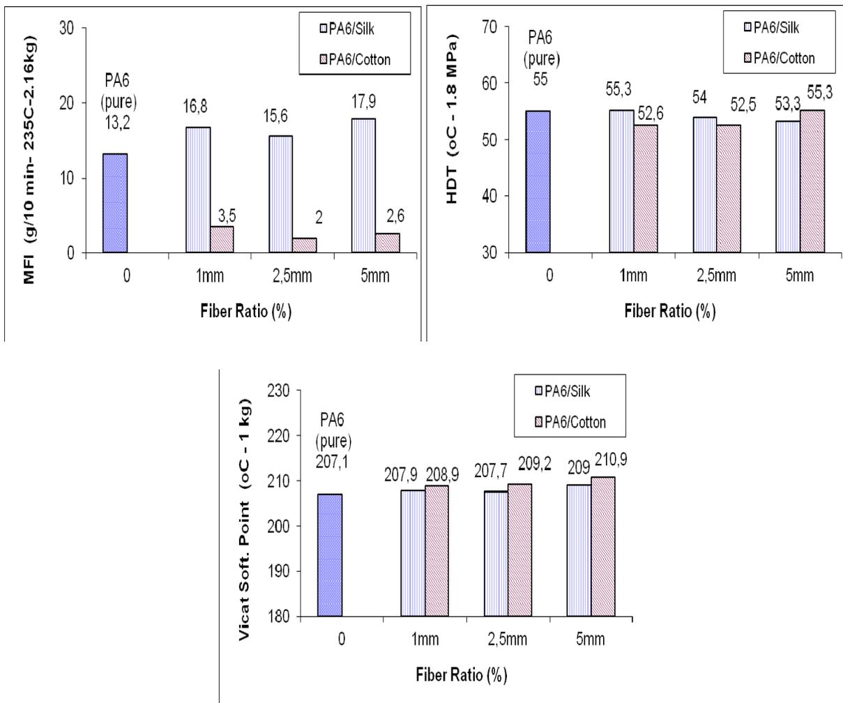
Figure 2 Thermal properties of the PA<sub>6</sub>/waste silk and PA<sub>6</sub>/waste cotton polymer composites
